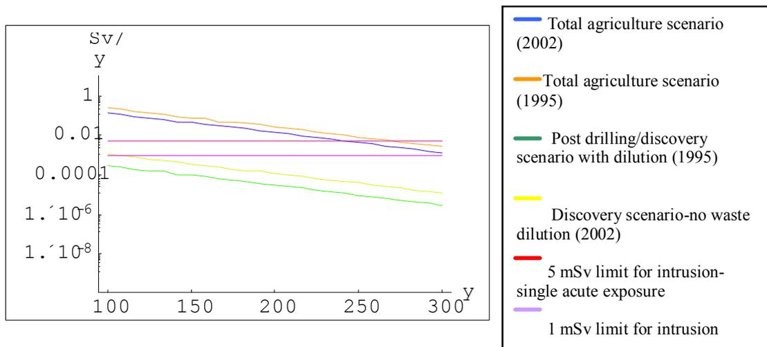
**Figure 19 – Concentration of Cs-137 below the repository when considered the retention of the unsaturated zone**
