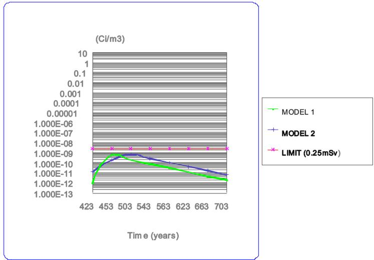
**Figure 14 –Maximum concentration in a well located at the bottom of the repository considering the retention on the unsaturated zone**
