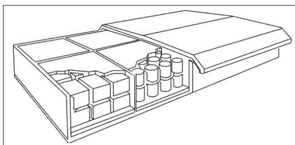
Figure 3 – Vault disposal facility type
