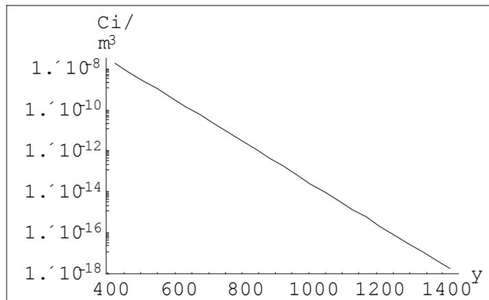
**Figure 18 – Concentration of Cs-137 below the repository when considered the retention of the unsaturated zone**
