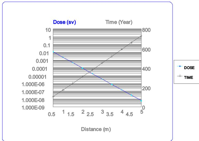
Figure 13 –Maximum doses as a function of the well distance
